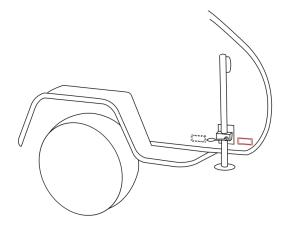
**2.** Place the fender box on the fender. Mark the 4 predrilled holes onto the fender and use a Ø8mm drill.
