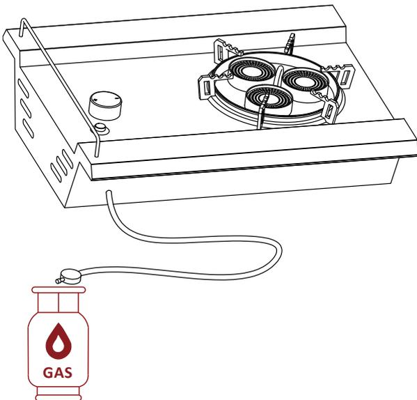
4. Press the ignition button and adjust to desired power.
