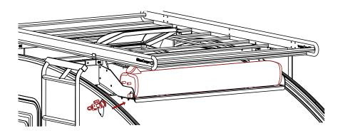
7. Mount the Water Hose. Ensure is clicks and are inserted properly. (Part used: F)
