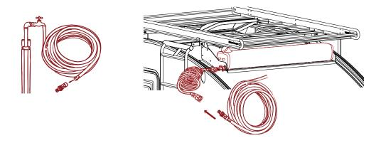
9. Finally mount the Water Spray Gun to the Water Hose. (Part used: E)
