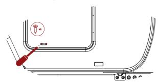
**7.** Drill the marked holes with Ø2.5mm drill. Do not drill deeper than 2cm.
