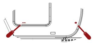
**3.** Use the hole without silicone to place the Magnet door holder.
