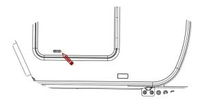
**5.** Mount Magnetic Door Holder with the 2 pan screws (TX20)
