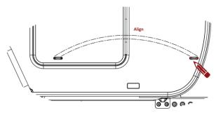
**8.** Mount the Magnetic Door Holder with the 2 pan screws (TX20)
