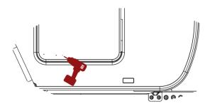
**6.** Align the other Magnetic Door Holder and mark the holes with a pen.
