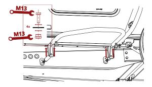
**6.** Adjust brackets with the nut using a M12 wrench. Tighten the locking nuts on each bracket to 25Nm with a M19 wrench.
