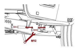
7. Mount the brackets to the chassis with 2x M13 wrenches. Tighten to 25Nm. Then repeat on the opposite side.
