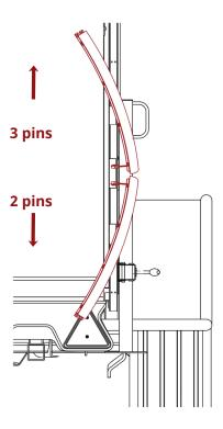
**17.** Mount the Zip-tie holders inside the U-profile. Fix the wire with zip-tie. (Part used: O, P and Q)
