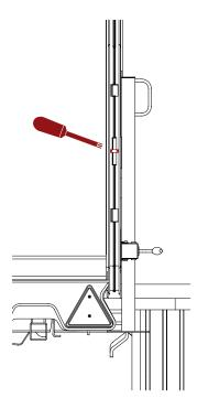
**5.** Cut the wires for clearance lamps on both sides of the terminals.
