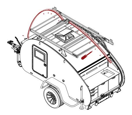
**13.** WARNING: Please make sure 2-3 person or approved lifting equipment that fits this procedure. Remount the rear door with the M8 hex key. Recommended torque is 14Nm.
