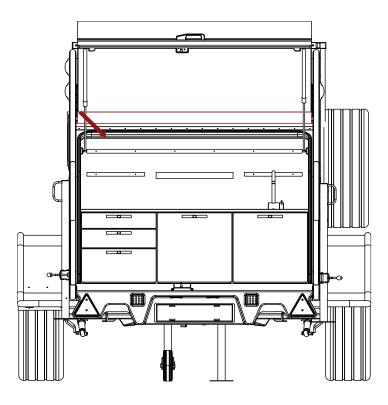
**9.** WARNING: Please make sure 2-3 person or approved lifting equipment that fits this procedure. The rear door will fall when gas damper is removed. Use M13 and M12 wrench to unmount the gas spring and keep the nuts for later.
