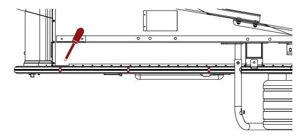
**7.** Unscrew all screws inside the U-profile and unmount the U-profile. If you only replacing the U-profile, please jump to Step 15.
