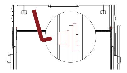
**11.** Unmount the screws on the L-profile. Unmount the L-profile and discard it.
