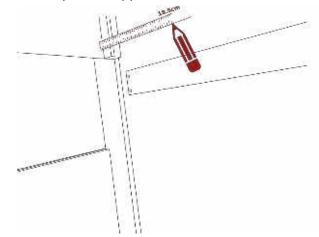
**3.** Measure from the floor of the camper and NOT the grid. Draw a line at 61cm from the 18.5cm mark and measure again 61cm about 40cm from the first mark. Use the leveling rule and draw a line between those 2 points. Repeat on opposite side.
