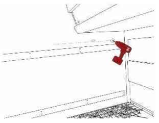
**5.** Place the rail(L/R) and then place the screw in the first hole. Before it is fully tightened, adjust the predrilled hole with markings with your line. Now mark the 5 remaining holes and drill as previous described. Repeat on opposite side.
