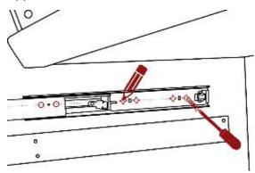
**6.** Start vacuuming to remove any shavings there may be on the rails. Place the bed on the rails. Insert the 6 bolts. Before tightening make sure the bed is correctly placed.
