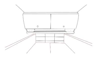
**2.** Measure from wall of the camper and NOT the cable tray. Draw a line at 18.5cm. Repeat on opposite side.
