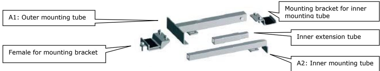
1. When mounting the suspension fitting from the Robot Trolley onto the caravan, start by gliding the two mounting tubes, A1 and A2, together, and then placing them up inside the side members.
