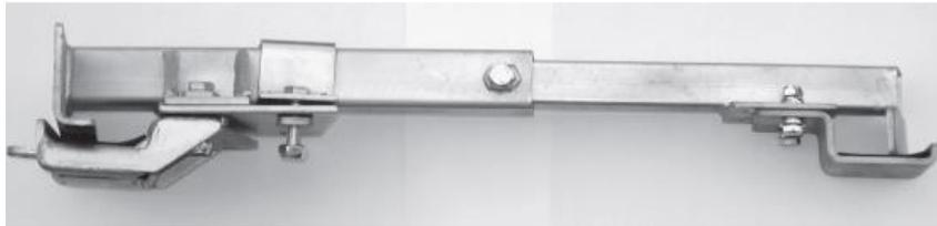
3. Slide the entire suspension fitting as far back on the side members as possible to put maximum weight on the Robot Trolley. Do not push the suspension fitting so far back that mounting and removing the Robot Trolley becomes difficult.
