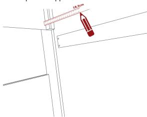
**3.** Measure from the floor of the camper and NOT the grid. Draw a line at 61cm from the 18.5cm mark and measure again 61cm about 40cm from the first mark. Use the leveling rule and draw a line between those 2 points. Repeat on opposite side.
