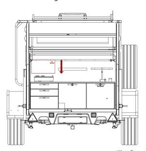
**2.** Always use a heat shield when using gas hob. We recommend storing the heat shield in the drawer while driving.
